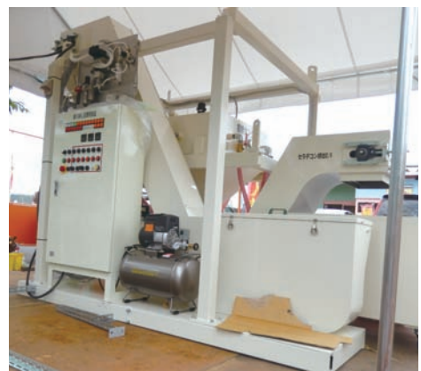
Facility for suppression of algal blooms
